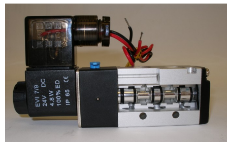
Figure 2: 4-way valve with cutout, showing piston.
